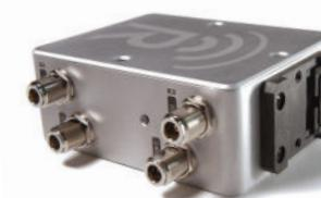
The BreadCrumb KM3 is intended for deployment inside pre-existing outdoor NEMA enclosures, featuring flexible DIN rail mounting to make deployments simple and fast.
