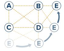
The Rajant mesh network quickly adapts to the changes caused by the movement of Node E. New resilient links are established in real-time keeping the network available, intact and secure.
