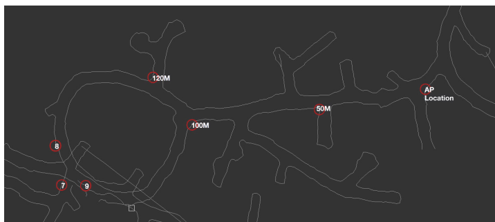
Onsite Test Locations, with minor and steep bends and turns (some more than 90 degrees), limited tunnel widths that have the potential to create severe Fresnel zone infringement, and a complete spiral.
