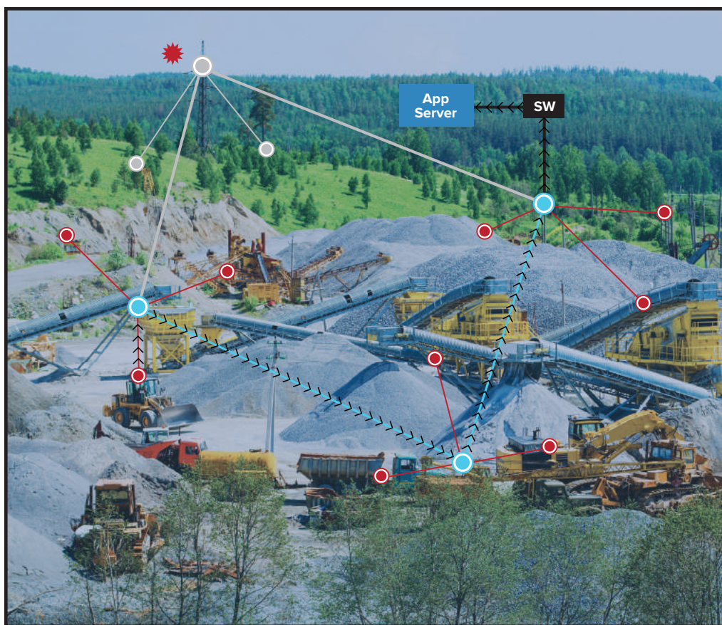
In a traditional wireless network as shown to the left, mobile nodes never communicate directly with one another. The mobile node transmits to its infrastructure node, and then the data has to travel either clockwise or counter-clockwise to get to the switch and application server. This slows traffic while increasing the potential for interference and congestion. Also, if an infrastructure node becomes unavailable, none of its mobile clients can access the network.
