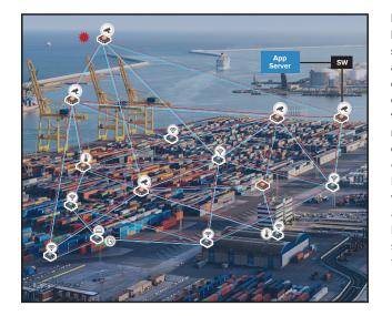
In a Rajant Kinetic Mesh network as shown to the left, any node can receive data packets from one peer and direct them to another via multiple simultaneous connections. This example shows BreadCrumb nodes with two frequencies, although each BreadCrumb can support up to four frequencies.
