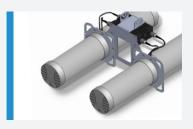
Rajant's RCP-2450 wide-band, circular polarized antenna system pairs with the Peregrine BreadCrumb to provide bidirectional coverage with dual frequency 2.4 and 4.9-5.85 GHz connections to assist in propagating signals around tunnel bends and to and from moving machinery.
