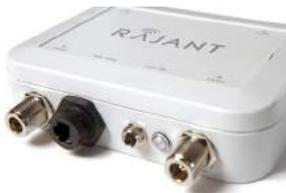
*The BreadCrumb ES1 is an IP67 device with multiple mounting options, making it ideal for deployment in and around pop-up triage centers and on mobile hospital surge units.*
