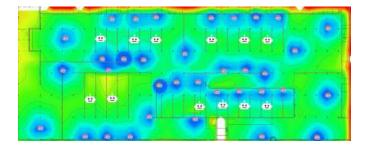
**Figure 2.** The solution to providing coverage for the entire floor of an indoor facility using a traditional enterprise Wi-Fi technology is to add in more nodes. The total number of infrastructure is now at 35 nodes to completely cover the area.
