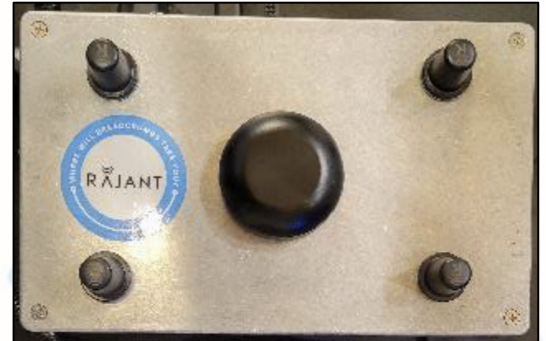
Ethernet Port - SAE Power Port w/ pigtail - Internal SAE connection - 3 amp inline fuse
