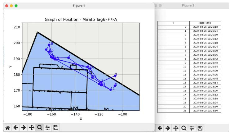
Same as to the left, with in addition the left hand side shows the location of the reference points (sGate gateways) next to the tracking map and the list of time stamps. What is interesting to show is that in the top corner of the plant there are only three gateways located approx. 45m / 150 ft. apart (on each tip of the contour of the plant) and the location of the forklift in that area (points 13-21) is precise and within the boundaries of the site
