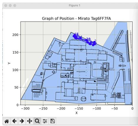
Track of a sTag associated with a forklift with related timelapse. Each geo-referenced position (numbered 1-21) is time stamped to keep track of the positions overtime. This data is available to export through Reios dedicated API and is used in Mirato business intelligence tool to perform analysis.
