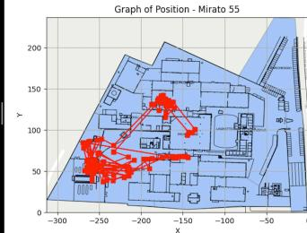
Two maps showing different ways to display the same data, i.e. historical positions of the plant guard with a sTag BLE badge. In Blue is just the superposition of all locations over a given period of time. Red is the superposition of all locations connected to reconstruct the actual path of the guard patrolling (static timelapse). Location captured every 6 sec, this is configurable
