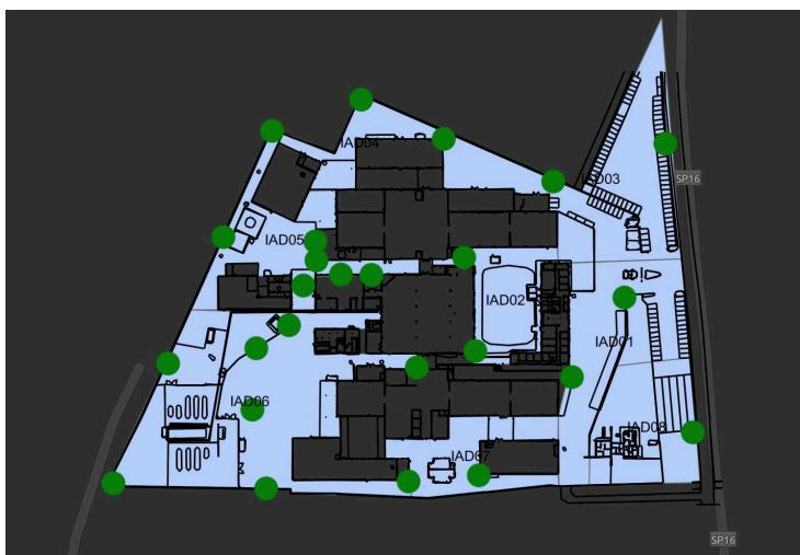
Live positions of the sGate gateways constituting the infrastructure to track the sTag associated to forklifts and personnel. All sGate are live (green dots). Some are mounted with the lighting fixtures and also perform lights control, others are placed standalone to enhance the coverage just for the tracking.
