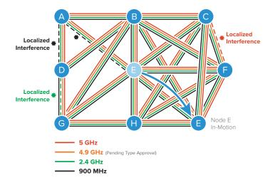
This diagram illustrates how a multi-frequency BreadCrumb network adapts to changes caused by the movement of BreadCrumb node E. New links are established in real time, keeping the network available, intact, and secure. The dotted lines show locations where radio frequencies experience interference. In such situations, InstaMesh instantly reroutes traffic over a clear frequency.
